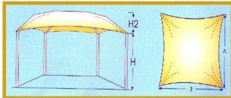
**CICOGNA** is the modular tent-covering, specially manufactured for car showrooms & car parkings. Its supporting framework is in Galvanized and white powder-coated steel & its covering is in a particular antirain and anti-hall elastomer PVC.
